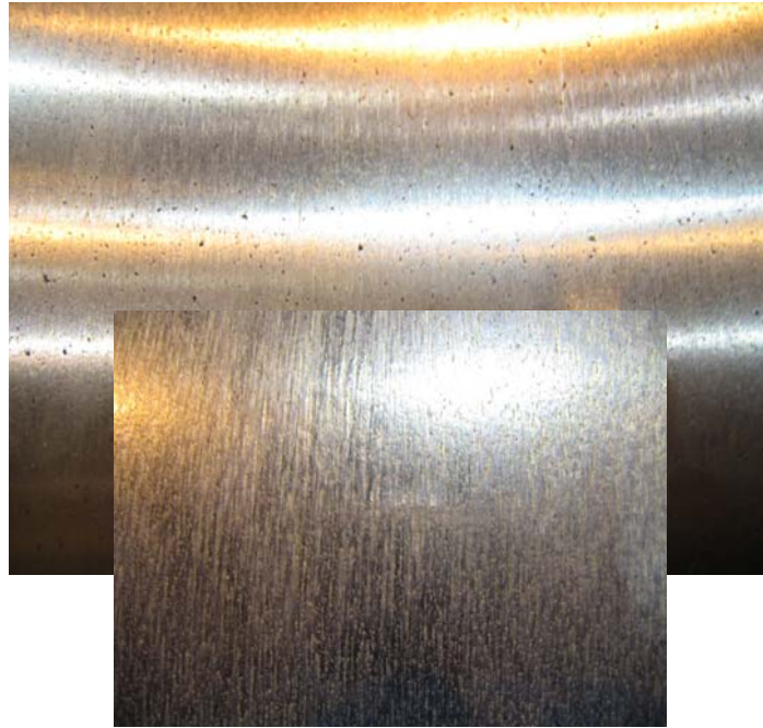
Figure 6 Pitting on the roll surface (Stand F1 after 10000 ton)
